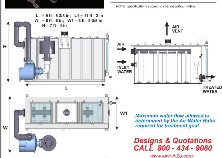
DEEPBUBBLE Multi-Stage Aeration Systems are furnished complete with blower, filter/silencer, and accessories with Lowry Aeration Systems' guarantee of performance. Optional control panels and booster pumps available.
