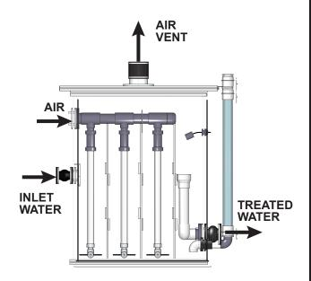
Maximum water flow allowed is determined by the Air:Water Ratio required for treatment goal
